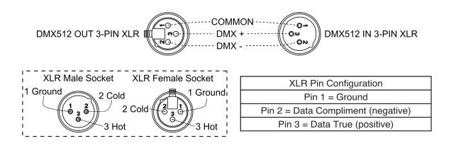
**Special Note: Line Termination.** When longer runs of cable are used, you may need to use a terminator on the last unit to avoid erratic behavior. A terminator is a 110-120 ohm 1/4 watt resistor which is connected between pins 2 and 3 of a male XLR connector (DATA + and DATA -). This unit is inserted in the female XLR connector of the last unit in your daisy chain to terminate the line. Using a cable terminator (ADJ part number Z-DMX/T) will decrease the possibilities of erratic behavior.
